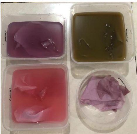
Fig. 2 Fixation Process, from upper left clockwise: Alum, \text{FeSO}_4 , without fixative, lemon juice. Source: Author's Documentation
